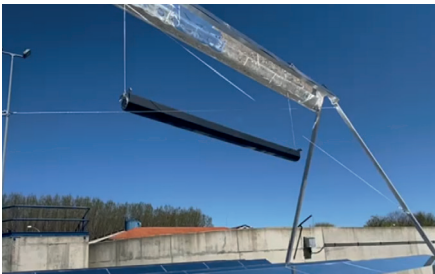
Channel receiver with hoisting system
