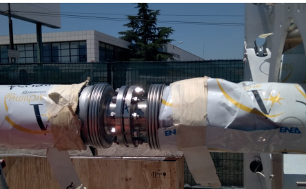
Connection between absorber tubes
