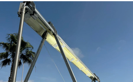
Transparent receiver in operation
